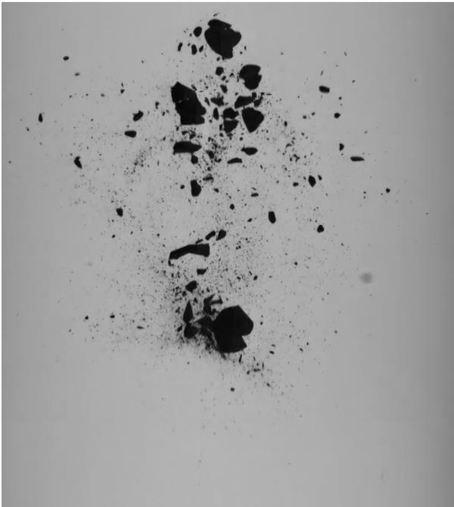
Silicate 2 cm dust aggregates 7.4 m/s relative velocity complete fragmentation
