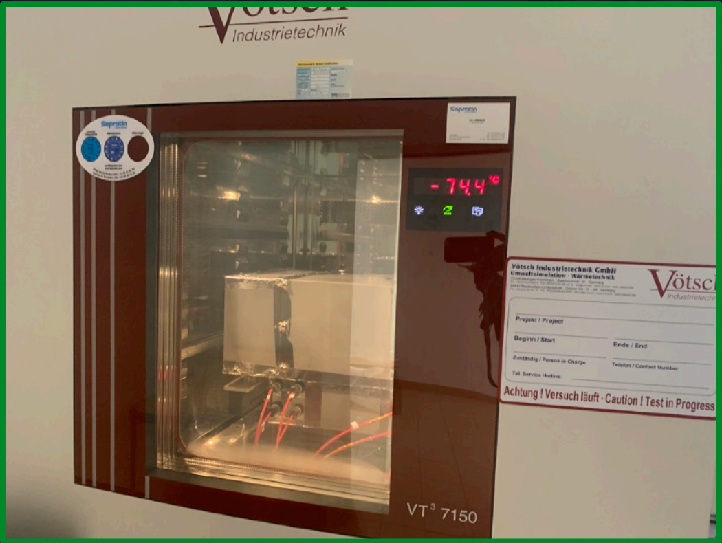
cold chamber tests @ -75°C
